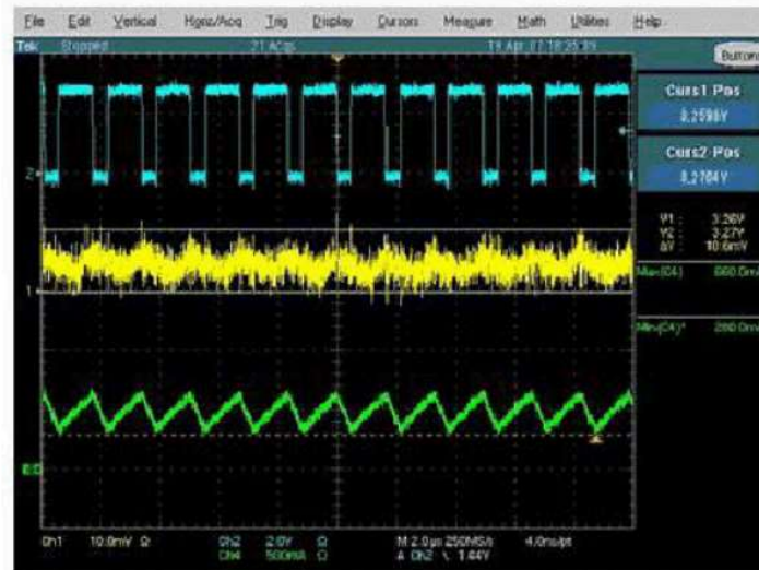
Figure 33. Ceramic 22μF 1210(X5R) (Good)
